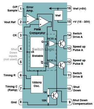
Fig. 3.4.3 The UC3524N (part detail)
