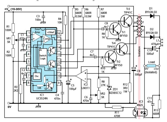
Fig. 3.4.2 Circuit diagram of a push-pull SMPS using the Texas Instruments UC3524 I.C.
