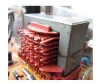
Fig. 3.4.6 Typical High Frequency Multi-Secondary Transformer
