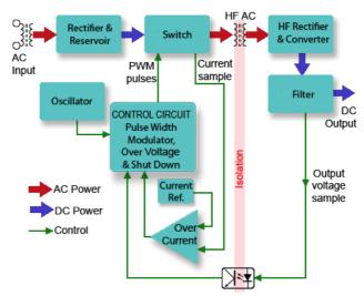
Fig. 3.0.1 Typical SMPS Block Diagram
