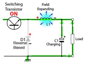
Fig. 3.1.2 Switching Transistor 'on' Period
