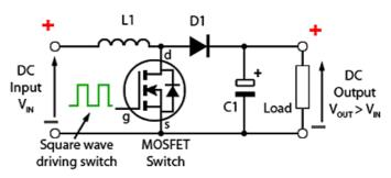
Fig. 3.2.1 Basic Boost Converter Circuit
