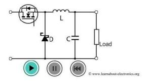
Fig. 3.1.3 Buck Converter Animation available at <a href="http://www.learnabout-electronics.org/PSU/psu31.php">http://www.learnabout-electronics.org/PSU/psu31.php</a>
