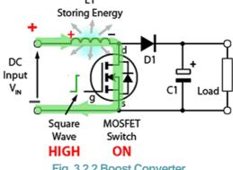
Fig. 3.2.2 Boost Converter Operation at Switch On
