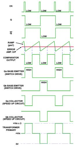
Fig. 3.4.4 UC3524N and Transformer Primary Waveforms
