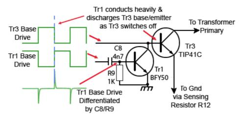
Fig. 3.4.5 Speeding up the Power Switch Turn Off
