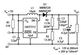
Fig. 3.2.6 Typical I.C. Boost Converter (LM27313)
