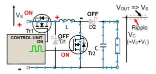
Fig. 3.3.4 Operation as a Boost Converter During Tr2 'on' Period
