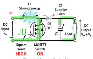
Fig. 3.2.4 Current Path with MOSFET On
