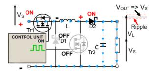
Fig. 3.3.5 Operation as a Boost Converter During Tr2 'off' Period
