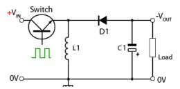
Fig. 3.1.4 Buck Converter for Negative Supplies
