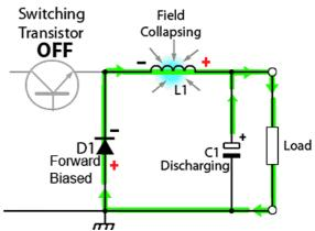
Fig. 3.1.2 Switching Transistor 'off' Period
