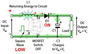
Fig. 3.2.3 Current Path with MOSFET Off
