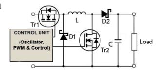
Fig. 3.3.1 Buck and Boost Converters Combined
