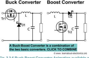
Fig. 3.3.6 Buck-Boost Converter Animation available at http://www.learnabout-electronics.org/PSU/psu33.php
